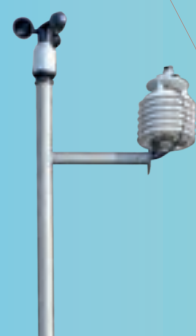
RTG control station with climate sensors (1802200)
