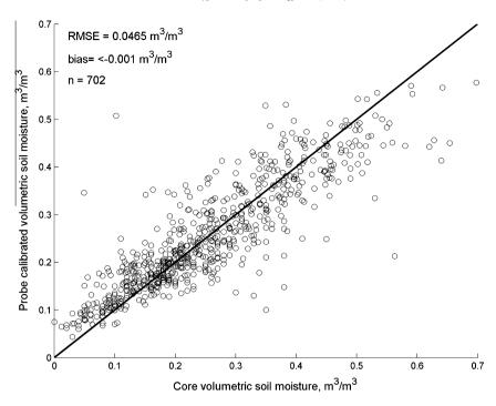
Fig. 3. Comparison of volumetric soil water content measured from the gravimetric core samples and the calculated volumetric water content using (6). The number of samples used in the establishment of (6) was 702. The solid line is the 1:1 line.
