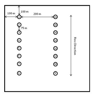
**Fig. 2.** Diagram of the manual soil moisture sampling transects. Sampling would begin at point 1 and progress in numerical order until point 16. The diagram is not drawn to scale
