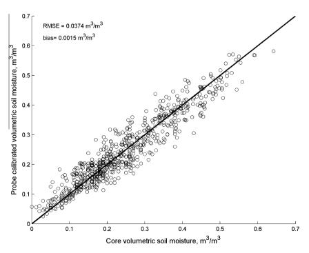
Fig. 6. Comparison of volumetric soil water content measured from the gravimetric core samples and the calculated volumetric soil water content, with individual field equations applied to data from the appropriate field. The solid line is the 1:1 line.
