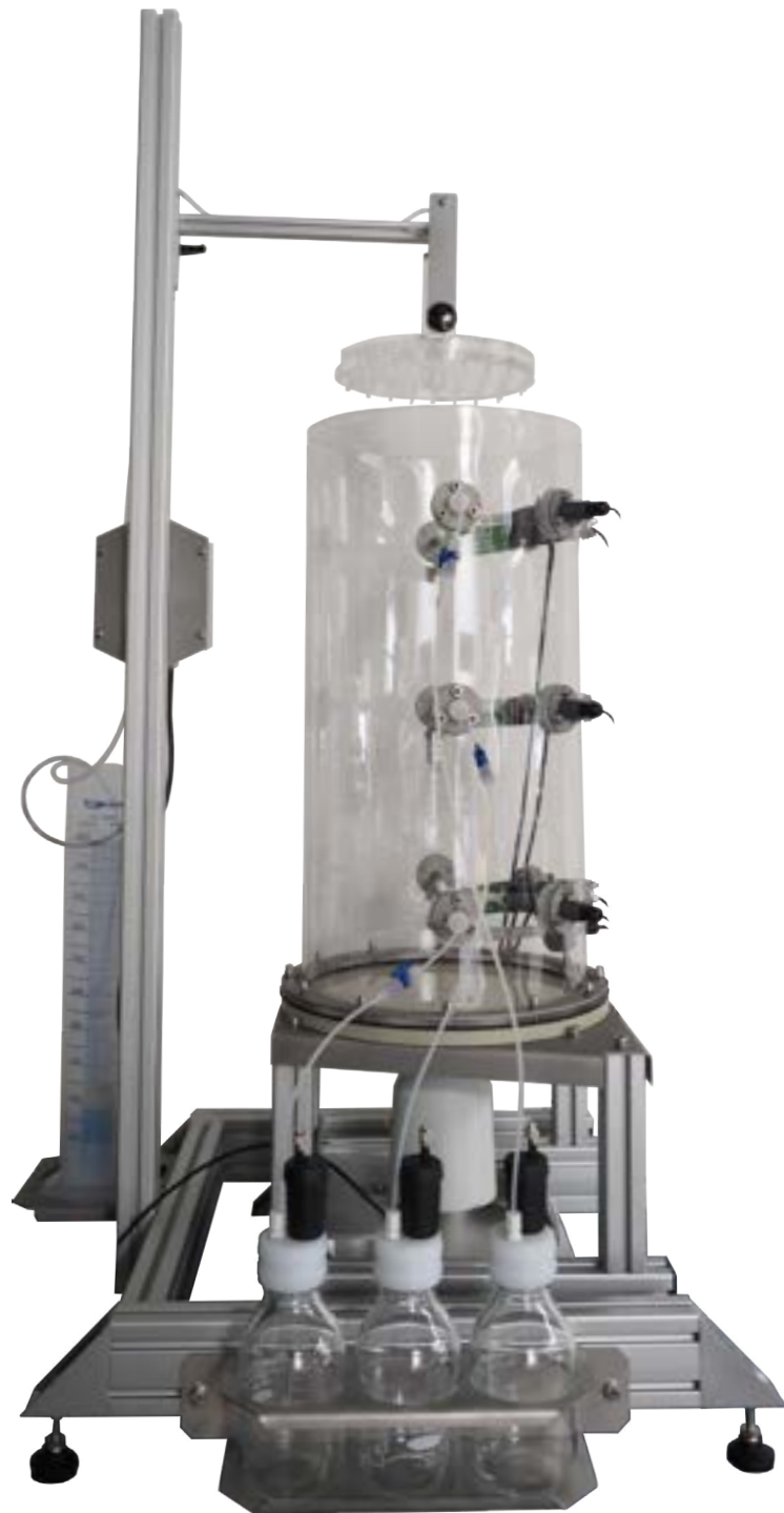
Laboratory lysimeter with PET lysimeter vessel
