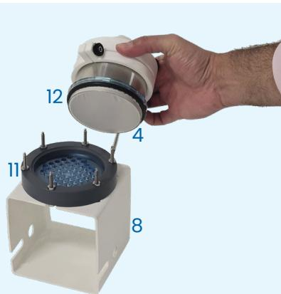
Mesh screen to hold soil sample in place allowing the exchange of water in and out of the sample
